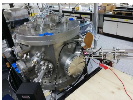
Vacuum chamber with discharge running on the right
