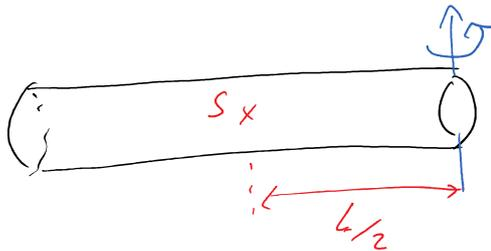
$$\begin{aligned} \Theta_{\text{Ende}} &= \Theta_{\text{Mitte}} + \left(\frac{L}{2}\right)^2 m \\ &= \frac{1}{12} m L^2 + \frac{1}{4} m L^2 = \underline{\underline{\frac{1}{3} m L^2}} \end{aligned}$$
