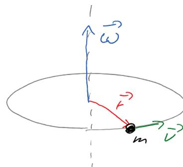
$$= \frac{1}{2} \frac{m r^2}{\Theta} \omega^2 = \frac{1}{2} \Theta \omega^2 = E_{\text{rot}}$$
