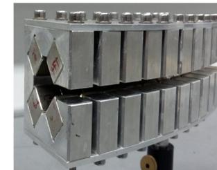
Picture of the quadrupole guide
