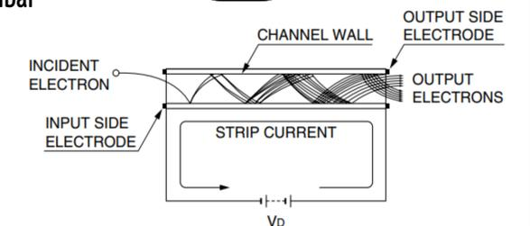
Structure and operating principle of the MCP [3]
