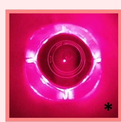
Absorption of hot bckg. + captured atoms measured
