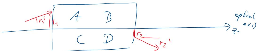
$$\begin{aligned} r_2 &= A \cdot r_1 + B \cdot r_1' \\ r_2' &= C \cdot r_1 + D \cdot r_1' \end{aligned} \quad \stackrel{\uparrow}{=} \quad \vec{r}_2 = M \cdot \vec{r}_1$$
