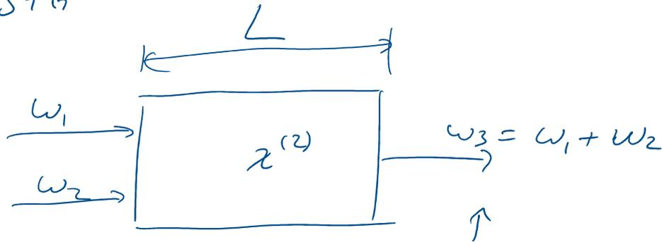
↑ electric field  $E_3$  at  $\omega_1 + \omega_2$
